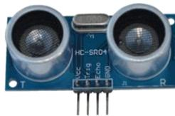
Gambar 4. 6 Sensor Ultrasonik
