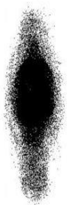
NOT ENOUGH AIR FLOW
