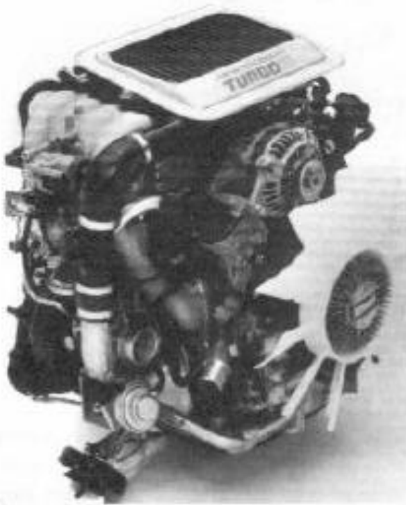
FIGURE 7.1a A turbocharged RX-7 rotary engine. (Photo courtesy of Mazda Motors of America.)
