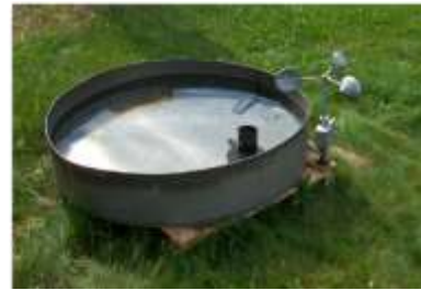
Gambar 6.9. Pan evaporimeter/ pan evaporation
