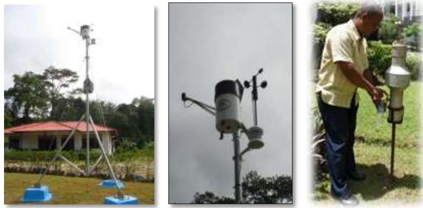
Gambar 6.4. Automatic Rainfall Recorder dan Ombrometer
