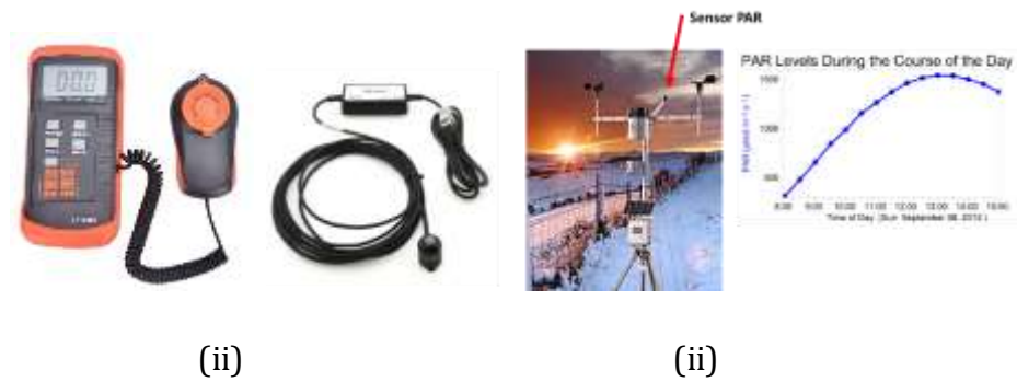
Gambar 6.8. (i) Digital Lux Meter (ii) Photosynthetically Active Radiation (PAR) sensor
