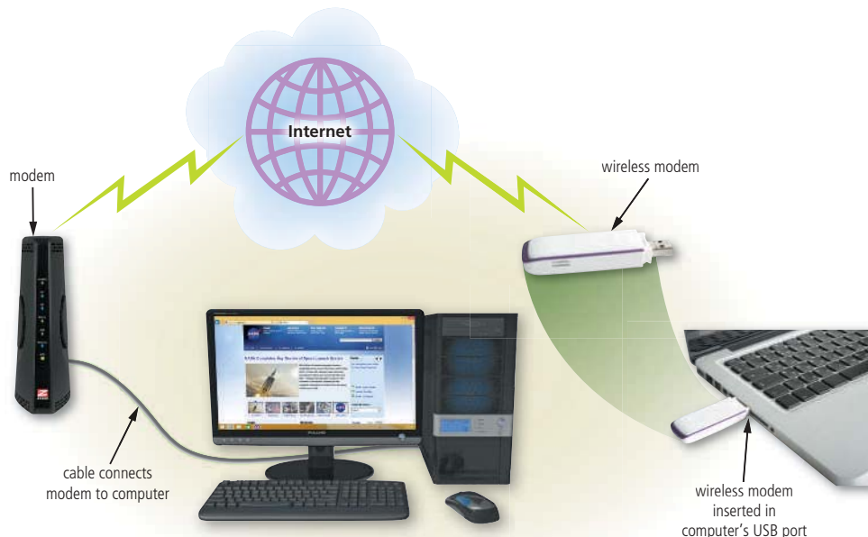
Figure 2-2 Using a modem is one way to connect computers and mobile devices to the Internet.
