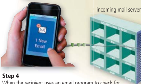
Figure 2-26 This figure shows how an email message may travel from a sender to a receiver.
