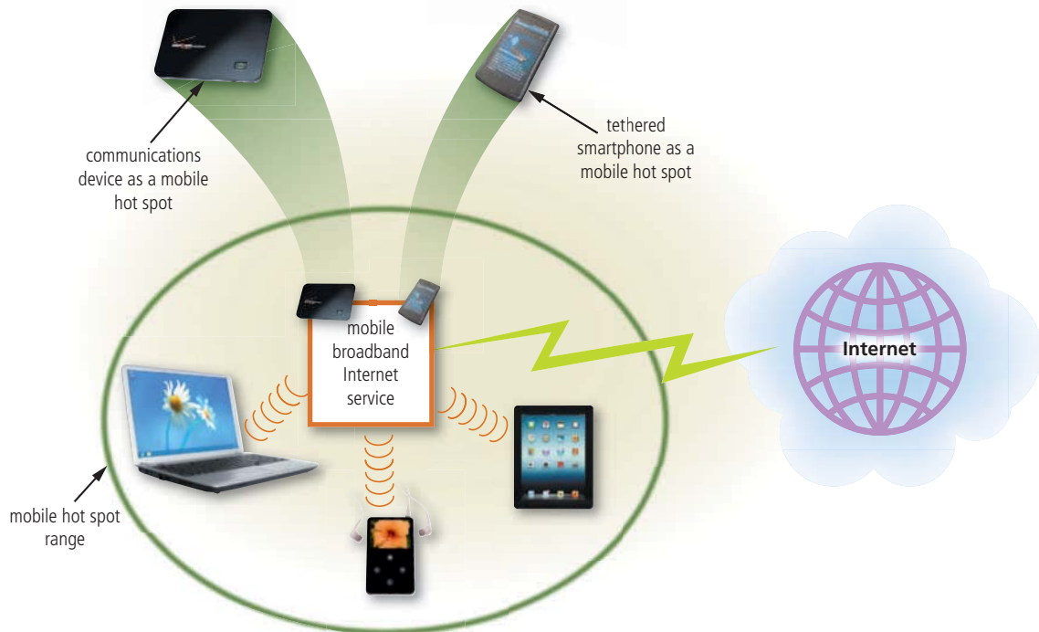
Figure 2-3 You can create a mobile hot spot using a communications device or by tethering a smartphone.
