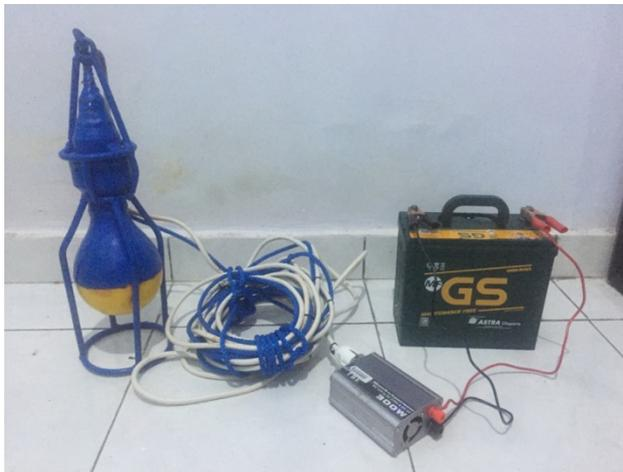
Gambar 2. *Light Aggregation Device (LAD)*
